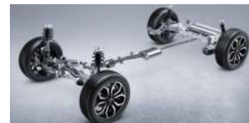
Rear Suspension Type Multiple link independent suspension
