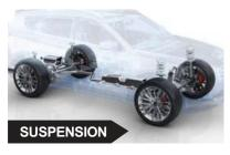
The multi-link suspension not only ensures the ride comfort, but also improves the tire adhesion due to the large number of links. It plays an important role in the driving comfort and stability of the car, and has become an excellent partner for JETOUR X70.
