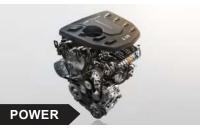
1.5T + 8AT Transmission (more fuel efficient due to more gears)
